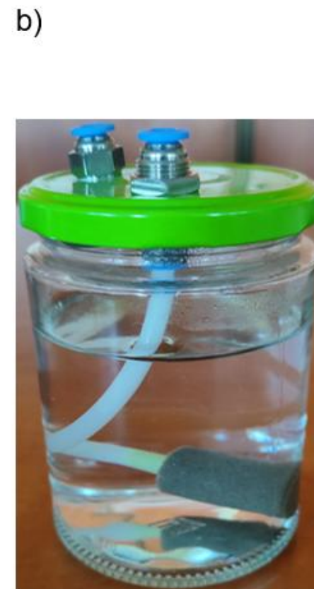
Fig. 5 Bubbler: a) 3D model – 1-glass jar, 2-screw cap, 3- pneumatic connector, 4-air stone, b) physical unit (model item numbers correspond to the actual components)
